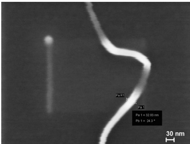
Fig. 4 Pristine MWCNTs with smooth surfaces
